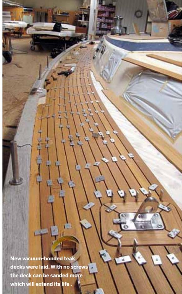
New vacuum-bonded teak decks were laid. With no screws the deck can be sanded more which will extend its life.
